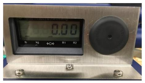
The weight displayed on the scale display is always the GROSS WEIGHT. The weight displayed on the main screen of the FairPick is the NET WEIGHT (Gross Weight – Tare Weight).
