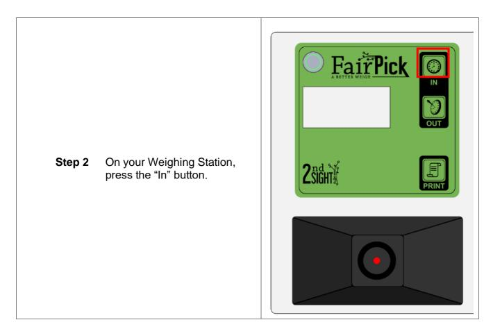
Step 3 Scan a Key Card by holding the card up to the RFID reader (the red light will be on in the middle of the reader)..
