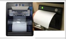
Step 8 For the auto-cut printer, press the "feed" and "cut" buttons to finish installing the new roll.
