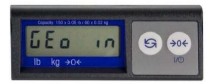
Note: The 7 segment display has limitations in displaying all alpha characters. For example, the letter "m" cannot be displayed, and will be replaced with an "n."
