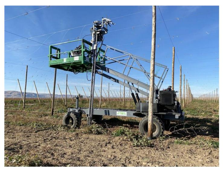
A Multi-functional Agricultural Vehicle operated by one person can twine hop trellises. The machine, built by 2nd Sight BioScience of Spokane, is being tested.
